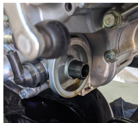
Oil Drained/Filter Removed
