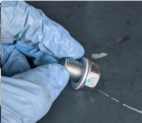
Clean Drain Bolt w/new crush washer
