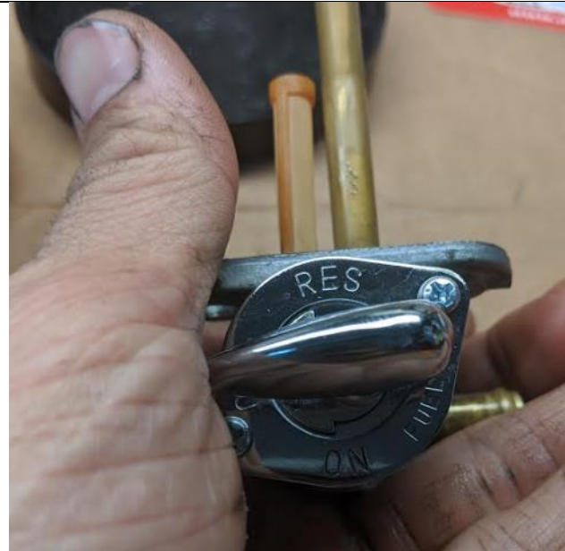
Petcock cleaned and rebuilt
