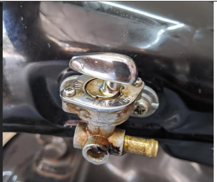
Fuel sender unit gasket requires replacement petcock should be rebuild with fresh gaskets
