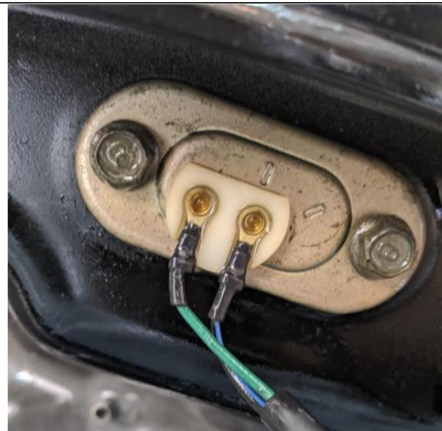
Fuel sender unit gasket requires replacement petcock should be rebuild with fresh gaskets
