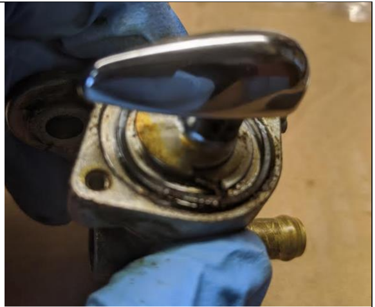
Gaskets needed to be replaced
