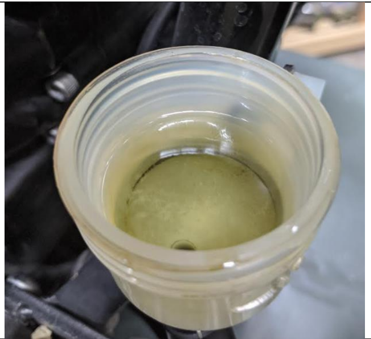
Bled and filled with synthetic DOT4
