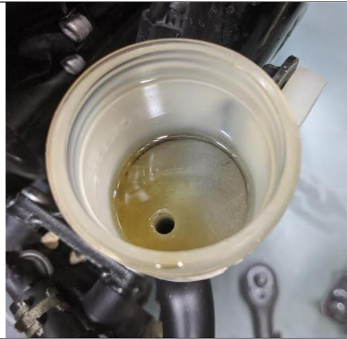
Rear brake fluid reservoir was empty
