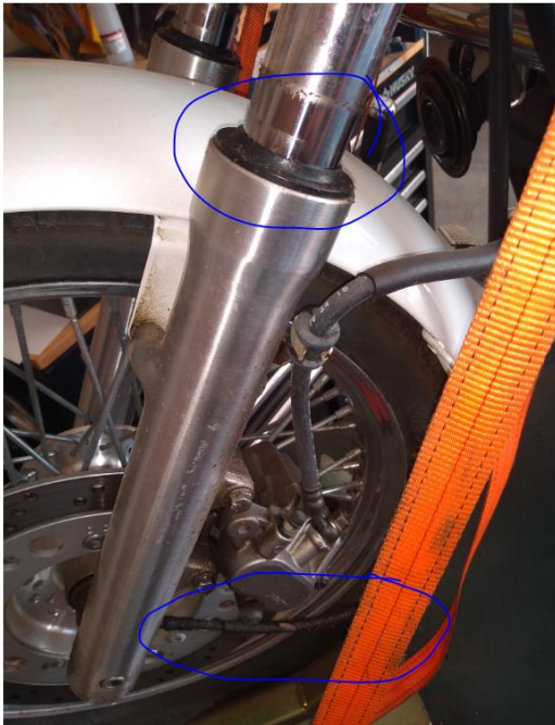
Forks show signs of leakage and oil residue on speedo
