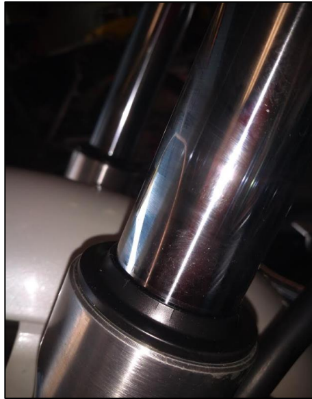
Oil Seals have been replaced
