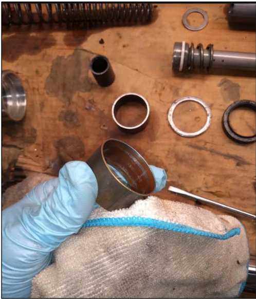
Fork bushings should be replaced
