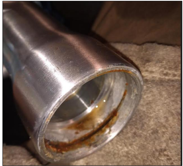
Right fork tube required extensive cleaning
