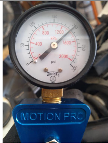
Rear cylinder Compression Test Results
